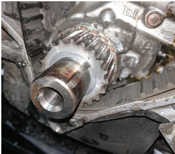
Failed Timing Belt
