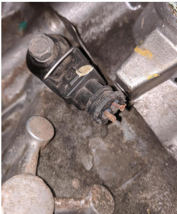
Knock Sensor Harness Damage
