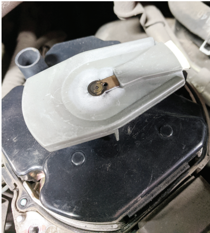
Worn Distributor Rotor
