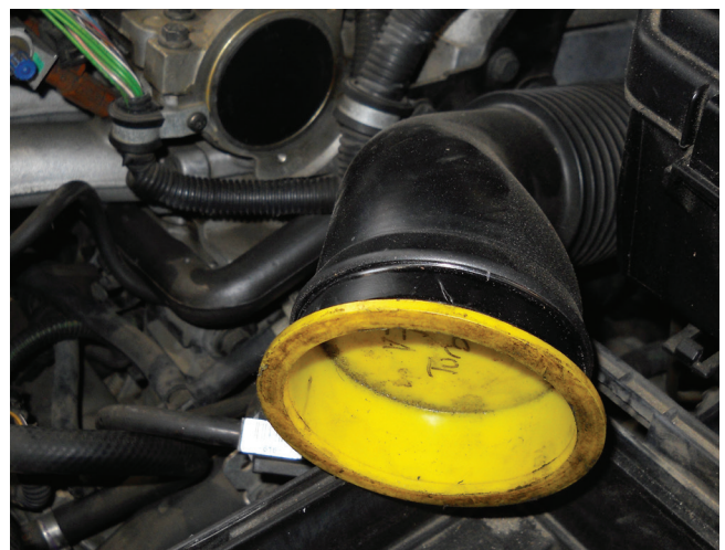
Air box pipe plugged for smoke testing
