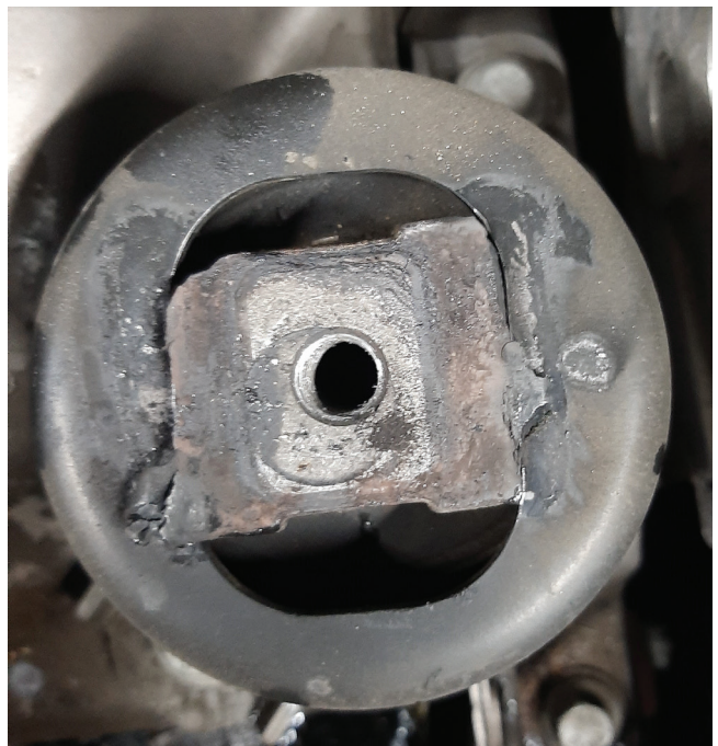
To confirm that the right hydraulic motor mount is worn out you may need to remove the upper mount bracket from the engine.
