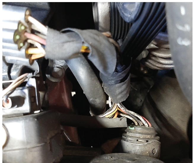
Belt rub damage to wire harness.
