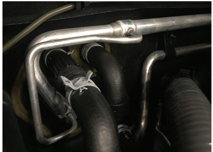
Internal heat exchanger
