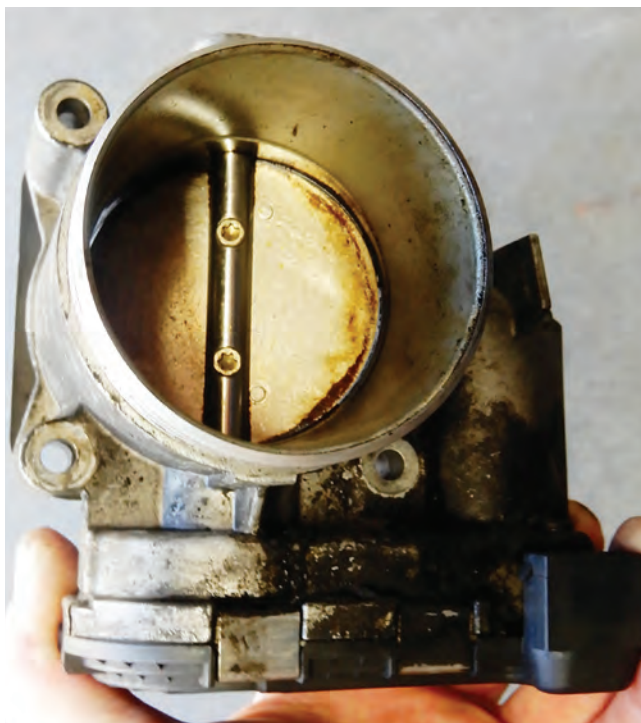
Electronic Throttle Module (ETM) that has been removed from vehicle, and throttle plate build up has caused the throttle plate to have resistance.
