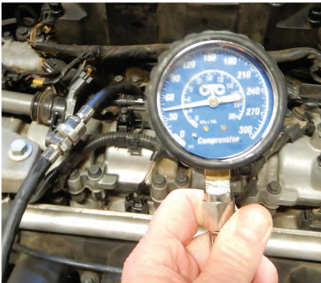
Taking a compression test on each cylinder to measure compression
