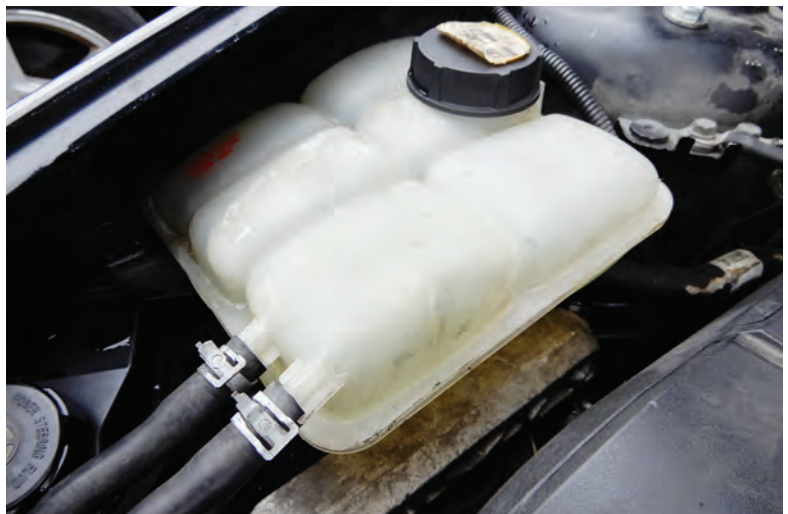
Coolant expansion tank back into place
