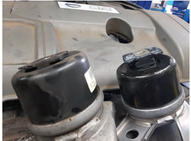
It's easy to see that the engine mount shown on the left is worn out when compared side by side with a new one, but this may be hard to see when the mount is still installed.
