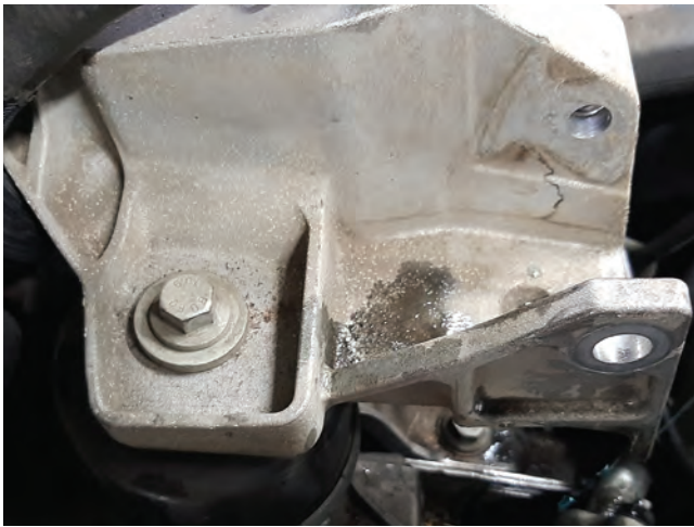
Top view of right mount bracket with torque mount removed.
