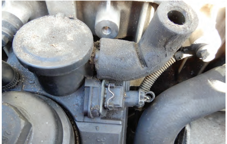
Plugging in electrical connector at oil filter housing
