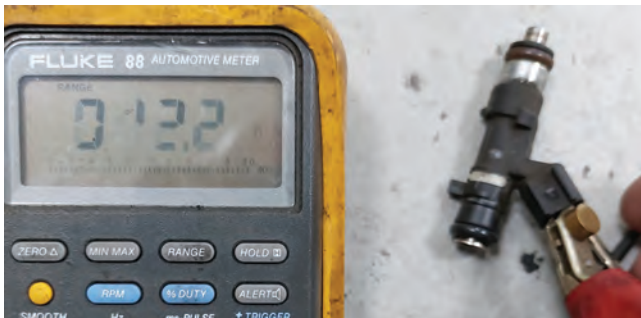
Old injector Ohm reading
