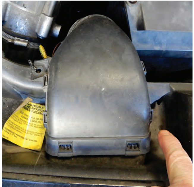
The two bolts that secure fresh air intake
