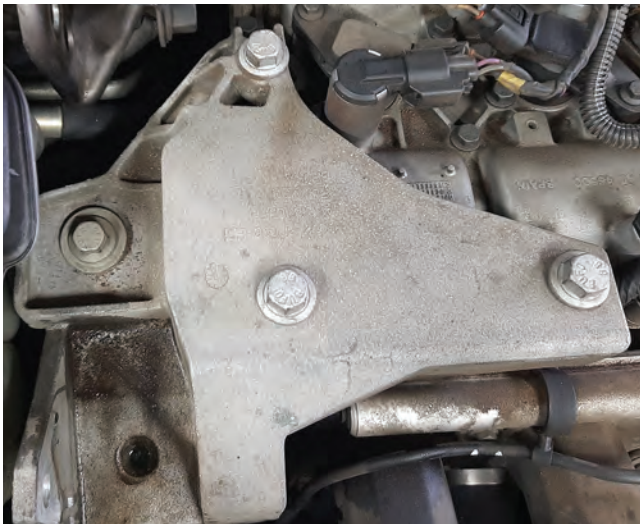
Top view of mount bracket with torque mount removed. This motor mount is hard to inspect without removing the upper engine torque rod and moving the coolant expansion tank out of the way.
