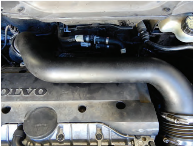
Hard pipe from air mass meter to turbo
