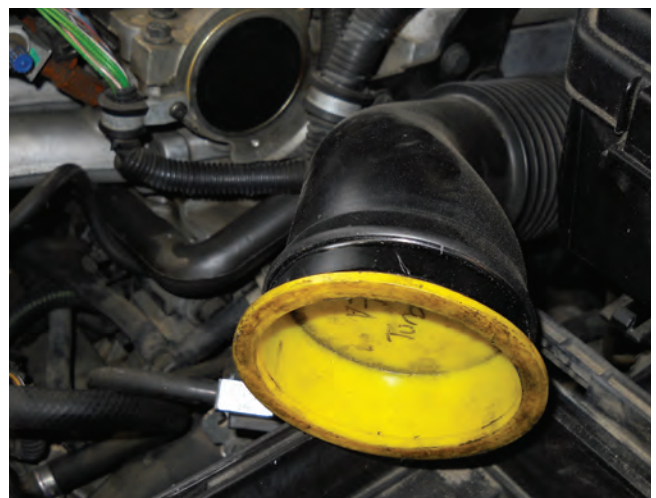
Air box pipe plugged for smoke testing
