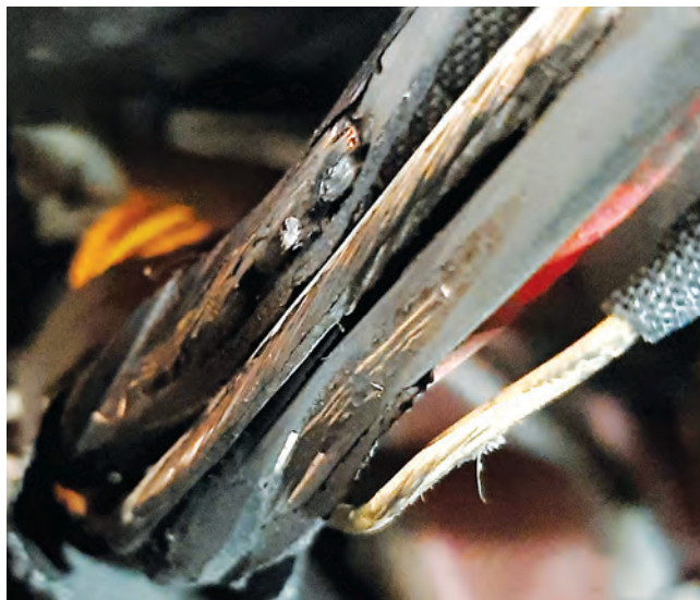
Belt rub damage to wire harness.
