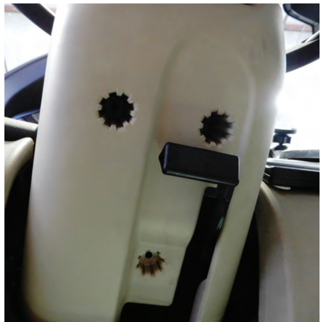
Trim around steering column needs to be removed
