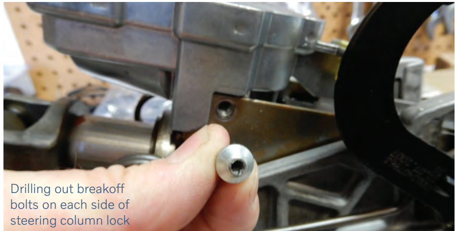
Steering column removed from vehicle
