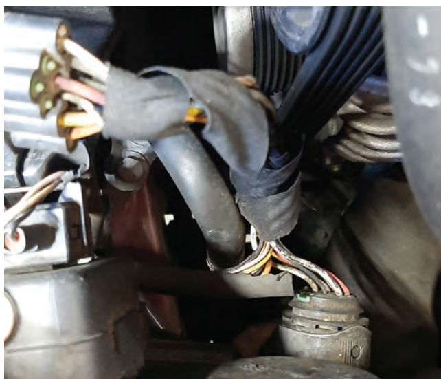
Belt rub damage to wire harness.
