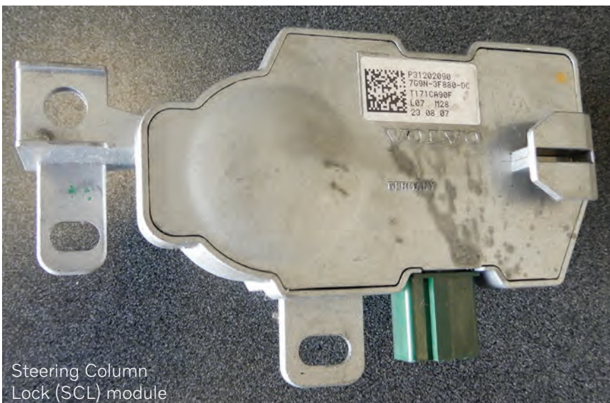
Steering column lock on bottom of steering column
