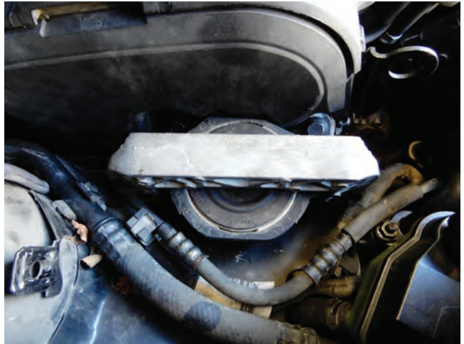
Front engine mount that needs to be removed
