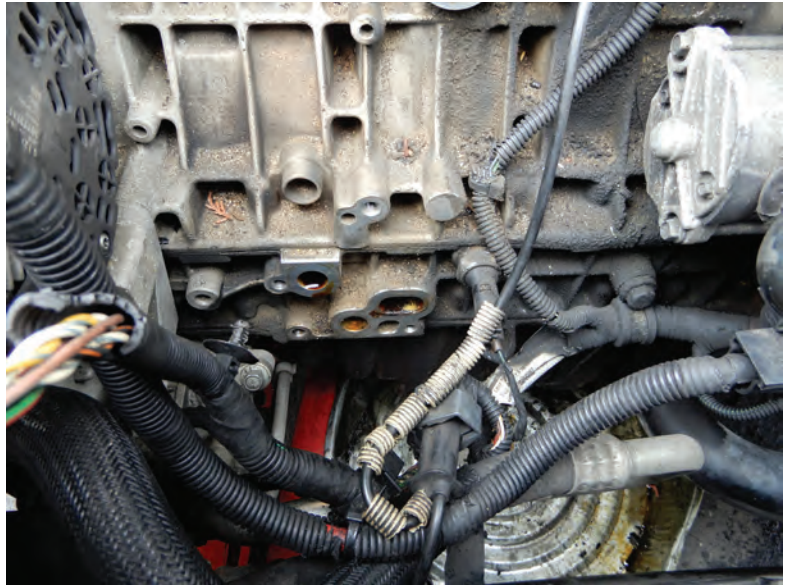
Oil filter housing removed from engine block and cleaned for new filter housing
