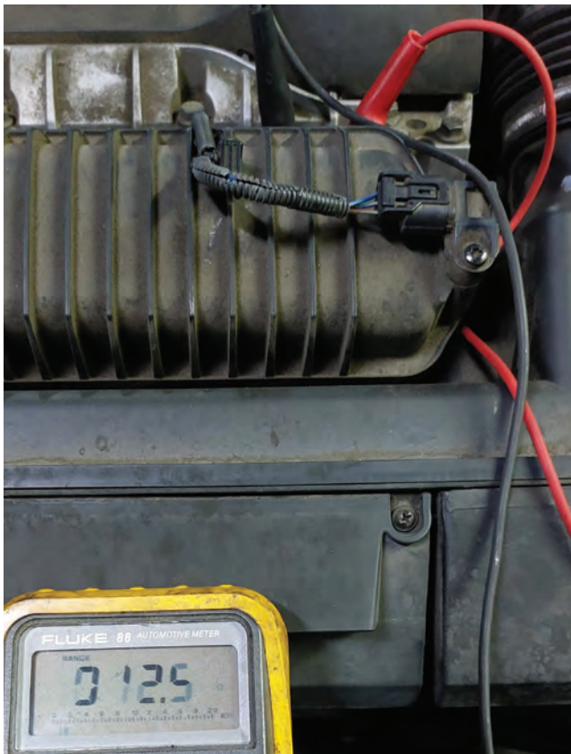
New injector Ohm reading
