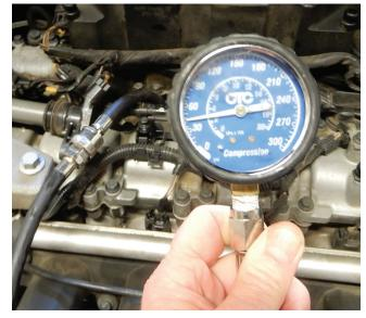
Taking a compression test on each cylinder to measure compression
