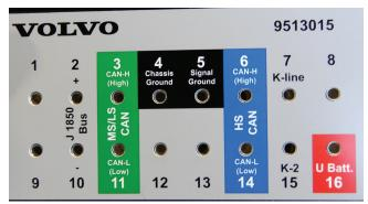
Special Volvo Tool number 9513015 hooked up to vehicle and checking voltage in the CAN System
