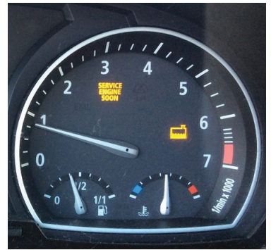
Low coolant level warning light
