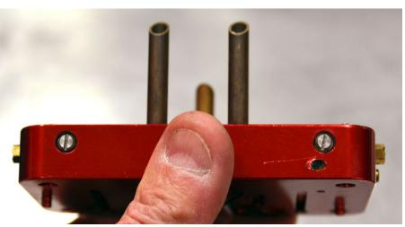
This is an interesting innovation from Willy's Carb Shop. The main jets are externally adjustable on this metering block. Brass tubes are inserted where the jets would normally be and there's a 5.5 mm, click-type nut just above the idle mixture screws on the side of the metering block with five positions from rich to lean. Pretty darned handy if you have to track-tune the main jets!
