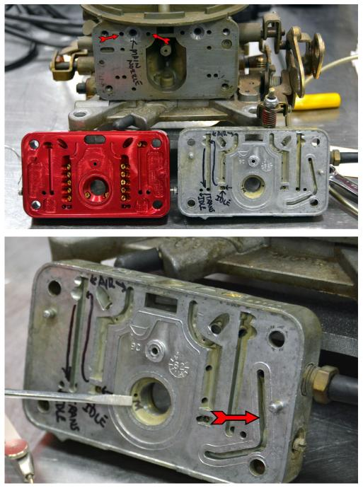
restrictor on the stock block to the right is a drilled brass insert, located at the lower end of the transfer/idle crossover channel. On the billet block, there's a screw-in restrictor just visible at the top of the channel in the pocket at the left of the main nozzle feed port. Replaceable jets make tuning much easier and can be reversed if you make a mistake.
