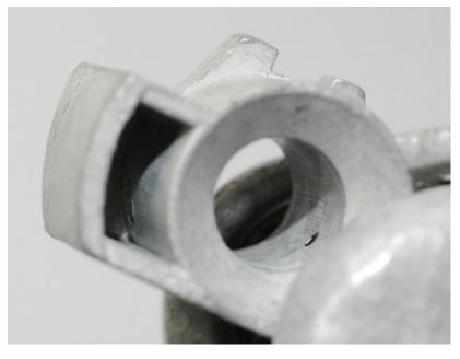
The anti-siphon or anti-pullover nozzle has a cup or guard that surrounds the nozzle so that air flow won't cause fuel to be pulled out of the accelerator
