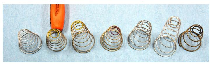
If you're running a vacuum secondary Holley, you may need to tune the opening rate of the secondary throttles. Holley makes a variety of color-coded secondary diaphragm springs to accomplish that. The chart will help get you in the ballpark, but if you notice, the spring opening RPM is displacement-dependent, so there's a little cut-andtry involved when you do your tuning.
