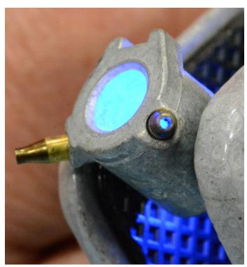
Tube nozzles are nice because they direct the fuel right at the booster, and they can be "aimed" a bit by carefully positioning them when you tighten up the mounting screw. They do extend out into the air stream, which can lead to pullover, so that's something to watch for if you are rich and can't find any other answer. Observing operation with loaded air flow may be the only way to catch a pullover problem.
