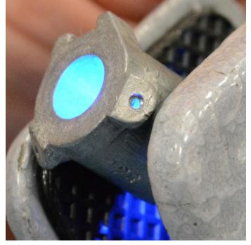
Above: A conventional or straight pump nozzle lacks the tube extension of a tube nozzle and the protective cup of the antisiphon. This is another part I used to drill, but now just buy the sizes I need because I discovered that if I drilled them to size sometimes the discharge stream pattern was thrown off. The other problem is once you drill them and then take them back out, you have no idea what size they really are unless you measure them.
