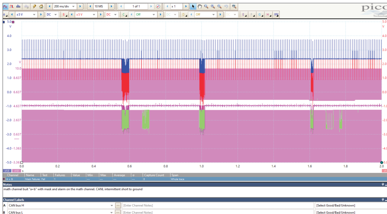
Figure 10: The Mask and Alarm strategy to catch CAN faults on the lab scope. The scope automatically captures and alarms the tech that the fault occurred. Not all scopes have this feature.
