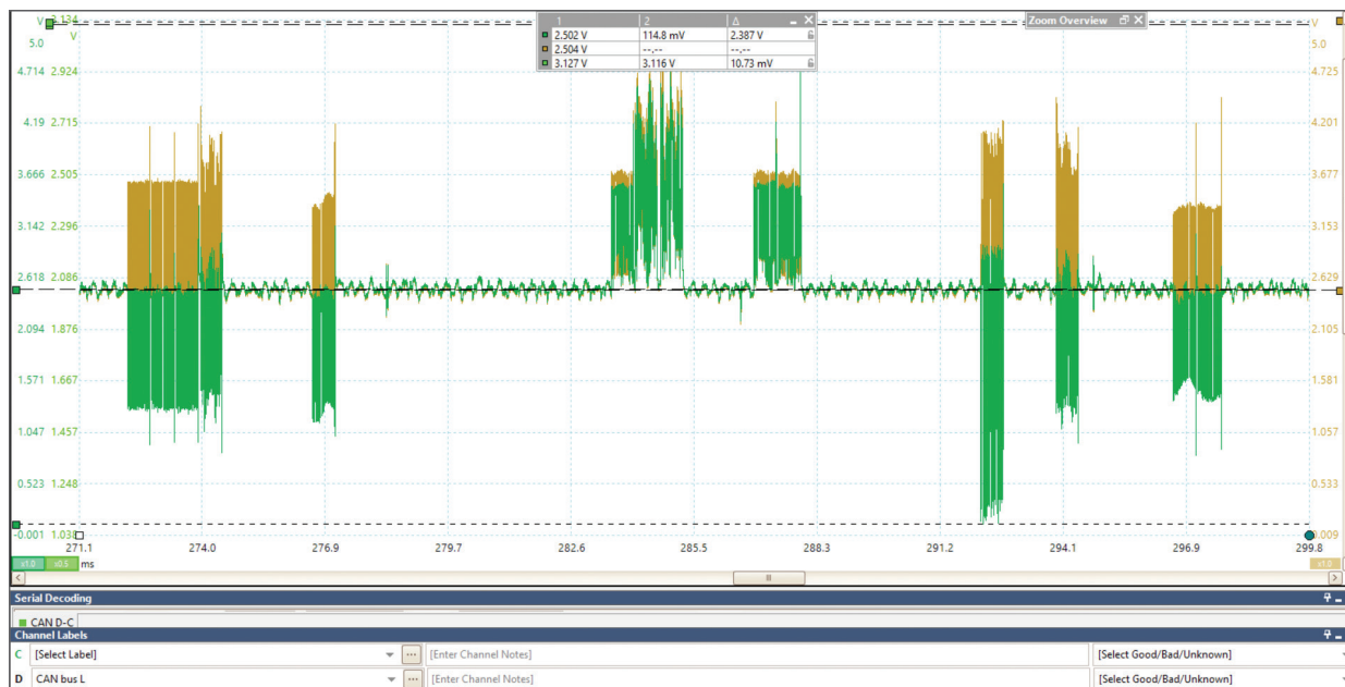
Figure 4: A zoomed in view of the CAN node losing electrical voltage control. Note that when this happens, the low bus signal covers up the high bus packets. Also note that during the fault, the node's signal is intermittently shorting to the power rail near 5v, and also to ground. The idle bus voltages appear to be fine.
