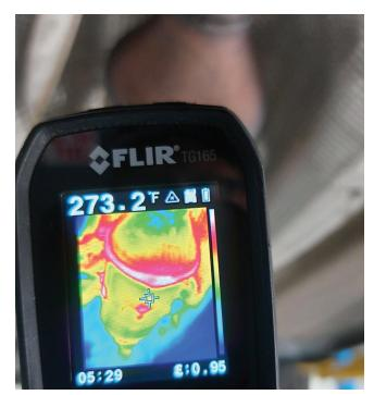
One really cool way of checking out the internal temperature of a catalytic converter as it warms up is to use a FLIR gun or FLIR camera adapter for your cell phone; you will be able to "see" the cat working. Possibly, but this is not always the case; testing is needed to determine the real cause of these codes.
