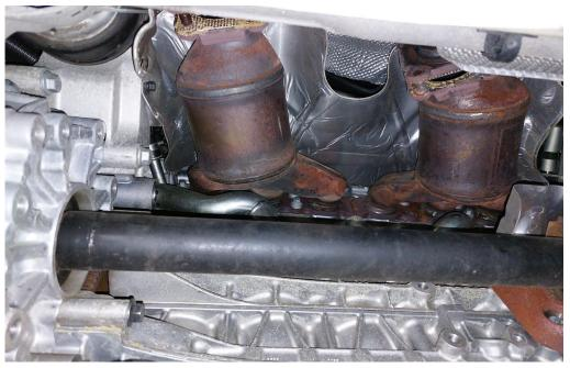
Volvo catalytic converters should last for the life of the car, but that's not always the case. Accurate testing is critical when condemning a Volvo converter because it can be easy to misdiagnose and you could replace a very expensive part and not fix the problem.
