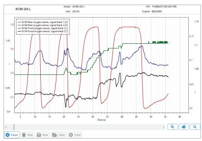
VIDA software is still the best tool to use when you are performing diagnostics like cat failure testing.
