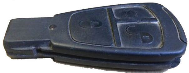
An original 1998-style DAS3 key. To switch between Global and Selective unlocking, press and hold both the lock and unlock buttons at the same time until the battery-check light flashes. To switch back, repeat the process.
