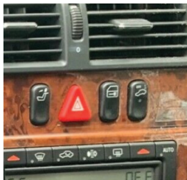
The interior central locking switch is to the right of the hazard flasher switch, and the rear head restraint release switch is to the left.
