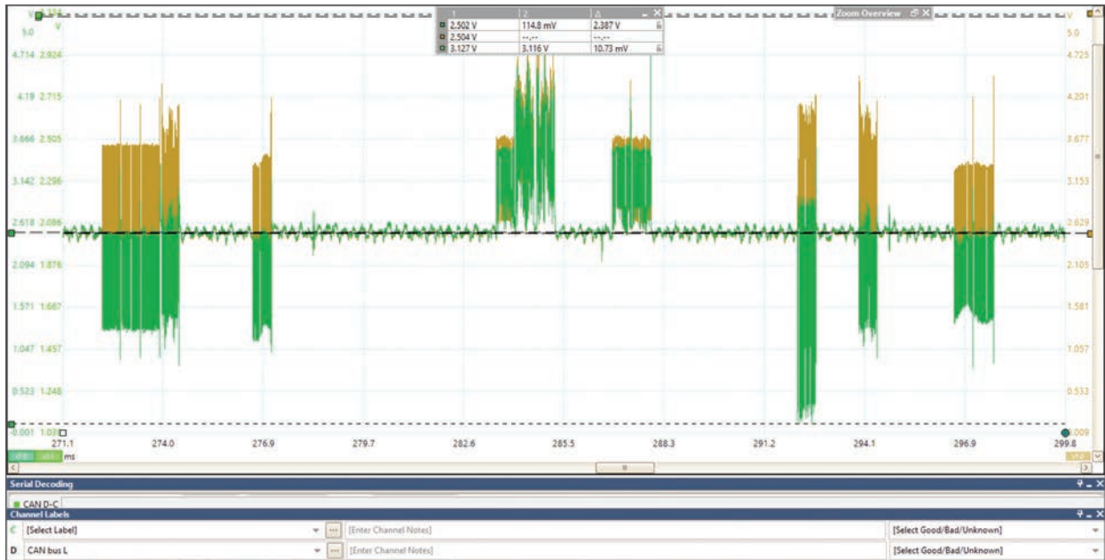
Figure 4: A zoomed in view of the CAN node losing electrical voltage control. Note that when this happens, the low bus signal covers up the high bus packets. Also note that during the fault, the node’s signal is intermittently shorting to the power rail near 5v, and also to ground. The idle bus voltages appear to be fine.
