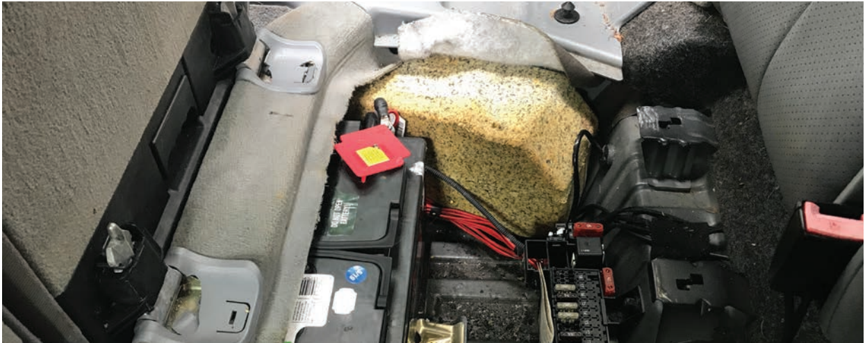
Hidden in that yellow foam block is the PSE unit, home of the central locking pump and other functions.
