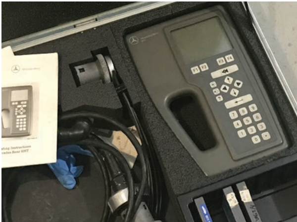
Now an antique, this hand-held Tester was the mainstay of vehicle diagnosis for Mercedes-Benz at the end of the 20 th century. Modern XENTRY Diagnosis systems can still fully diagnose HHT-based vehicles.
