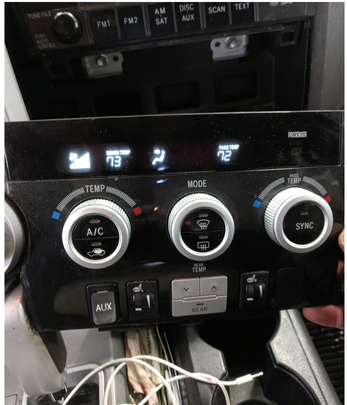
Sequoia HVAC Control Panel
