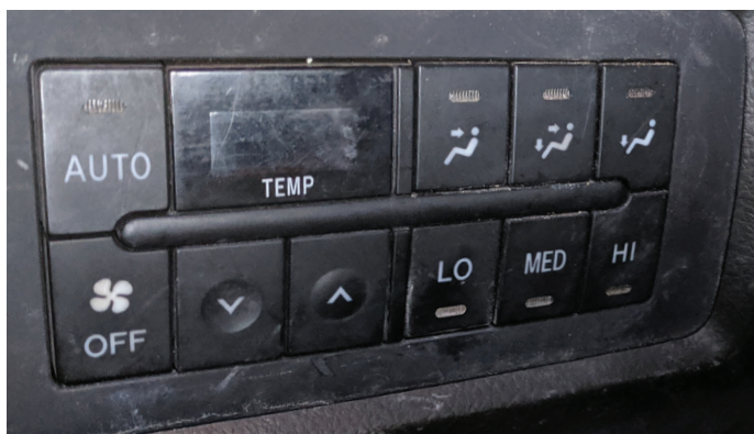
Rear HVAC Control Panel
