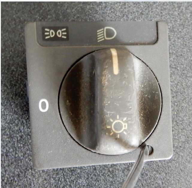
Headlight switch with adjustment to shut off daytime running lights
