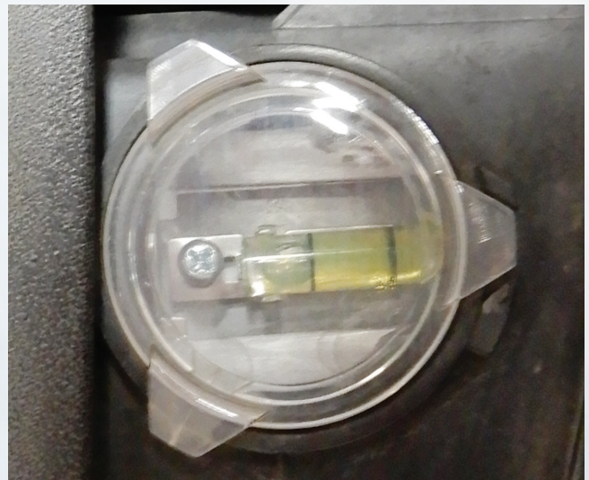
Small bubble adjustment on top of headlight assembly
