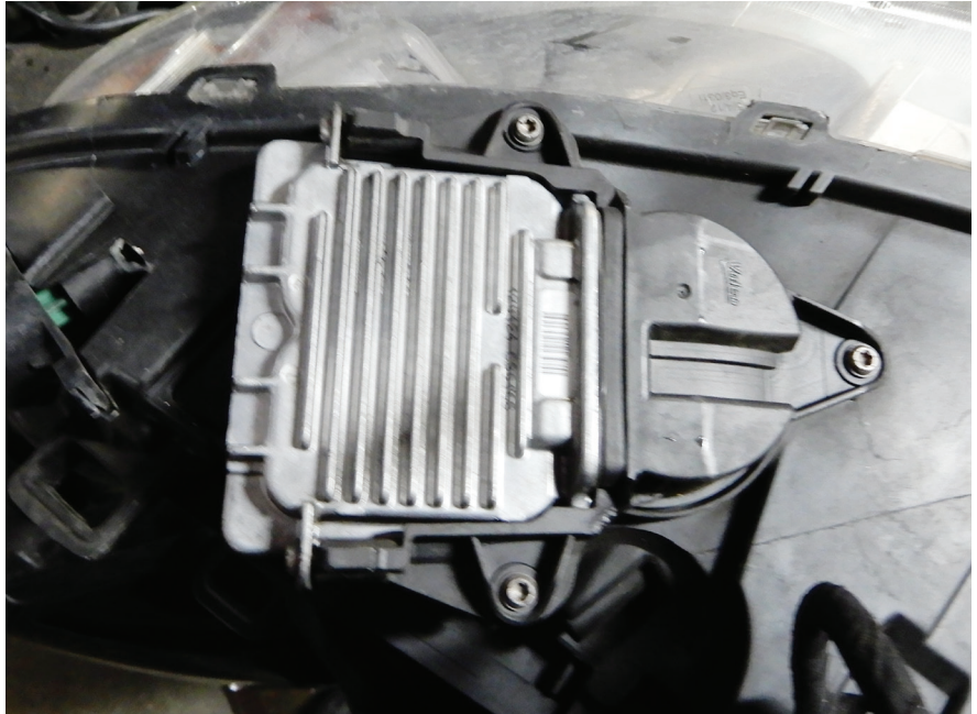
The basic ballast that is positioned on the bottom of the headlight assembly
