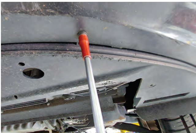
Remove T25 screws under the bumper cover.
