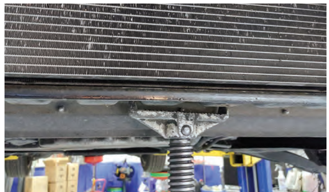
Support the radiator assembly with a jack stand.
