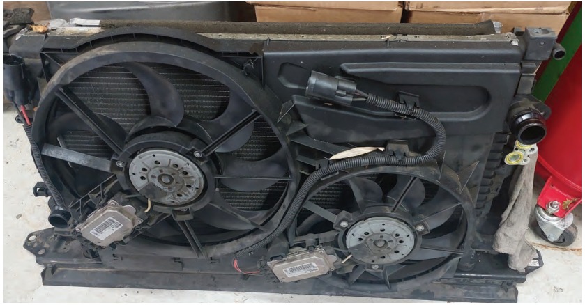
You can take out the fan assembly, A/C condenser, and radiator as one unit; this will save you a lot of time and a lot of extra work.
