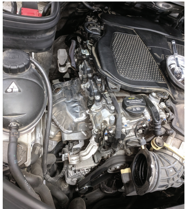
The right cylinder bank in a GLK350
