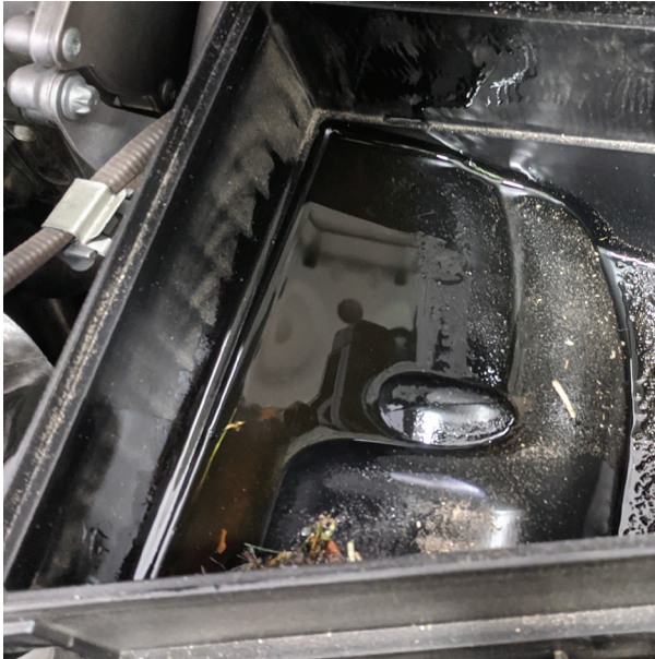
Oil pooled in the air cleaner housing
