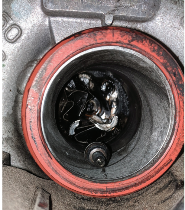
Failed Sprinter van turbocharger
