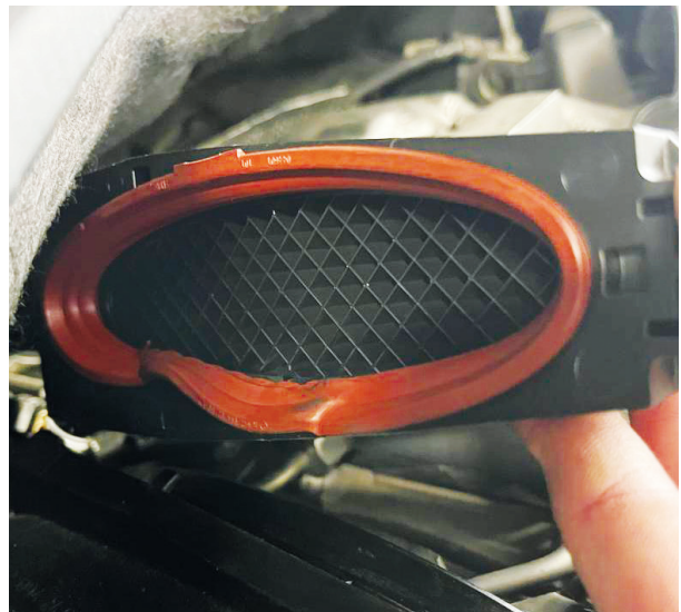
Deformed charge air pipe seal
