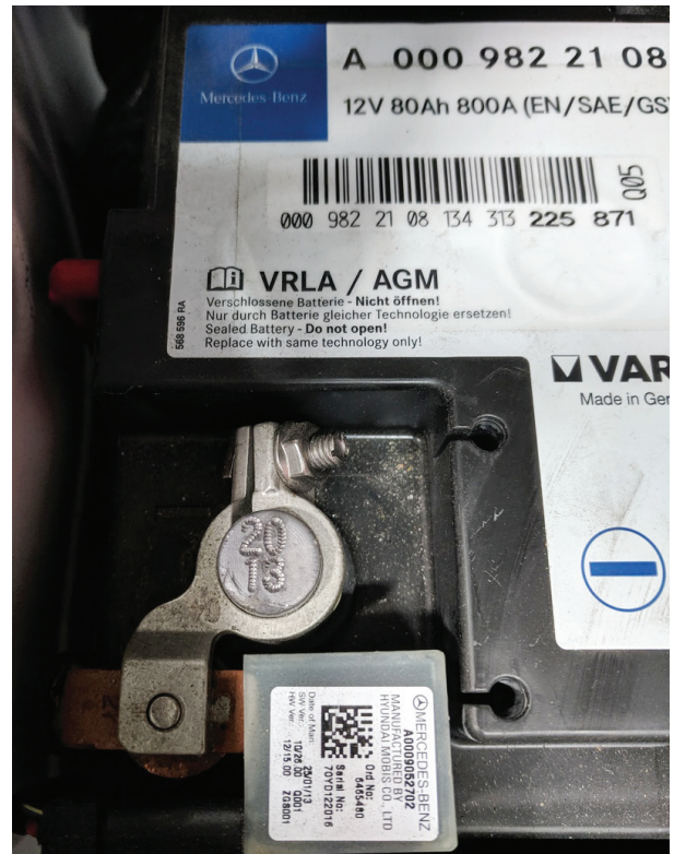
The battery terminal date code can be stamped on the negative post, or found on a label.
