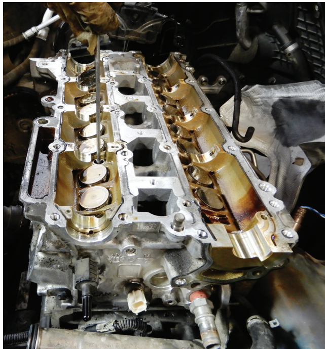
Removing valve tappets using a magnet
