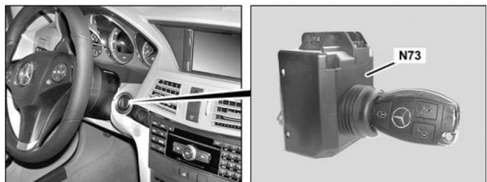
Figure 1: The Electronic Ignition Switch (EIS, N73) which uses IR signaling to 'talk' with the key and RF to supply power to the key. See the Mercedes-Benz Workshop Information System (WIS) for system description and operation, which differs by year and model.
