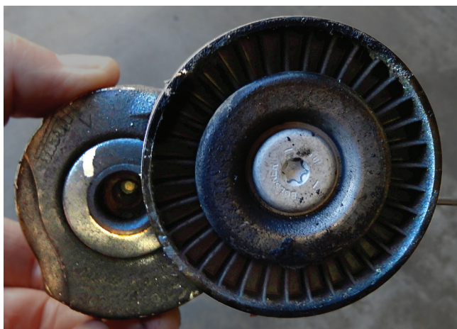
Belt tensioner with 3 mm pin in place
