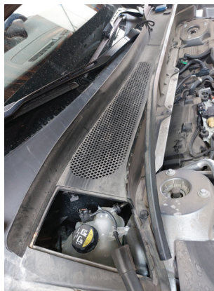
Remove cowl to expose the crossbar and wiper motor assembly.
