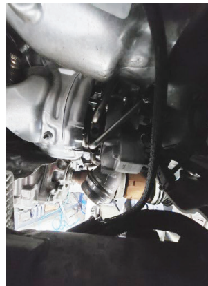
With the right inner fender covers removed, you will gain more access to the area.
