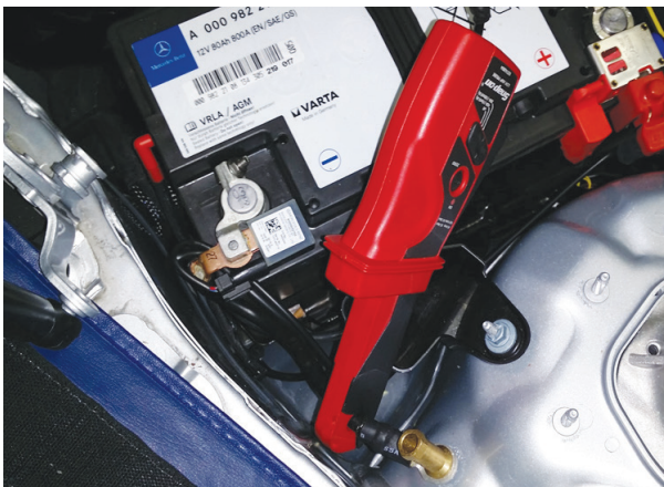
Use a clamp-on current probe to monitor the current on the negative battery cable.
