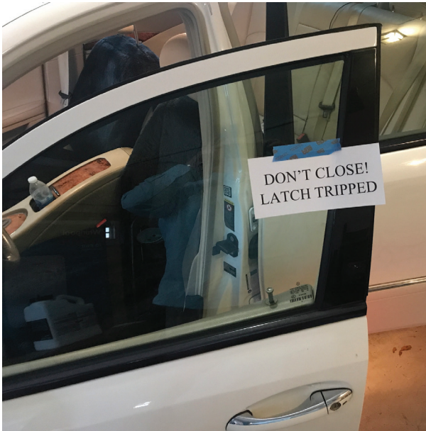
In our shop, we put a paper sign on each latch to help avoid lock damage.
