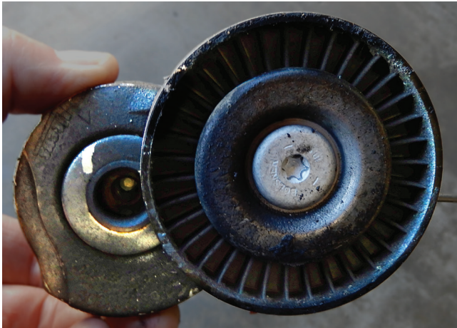
Belt tensioner with 3 mm pin in place
