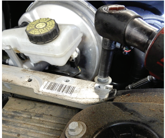
Aluminum crossbar that needs to be removed
