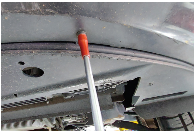
Remove T25 screws under the bumper cover.
