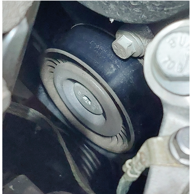
Remove auxiliary belt idler bearing after right motor mount is removed.
