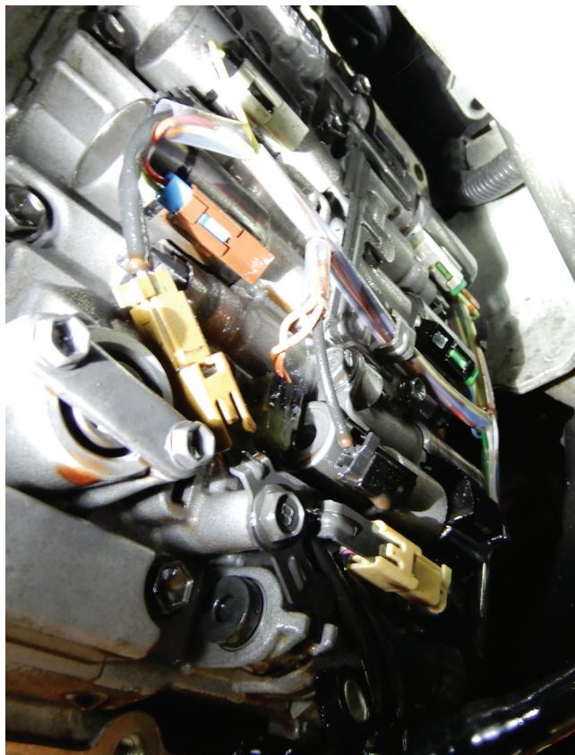
Valve body and solenoids inside transmission
