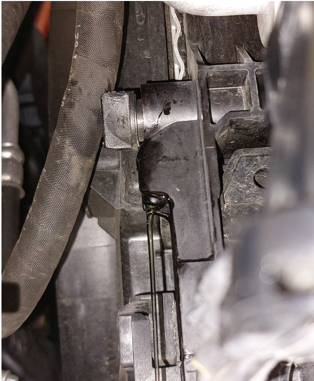
Radiator drain cock
