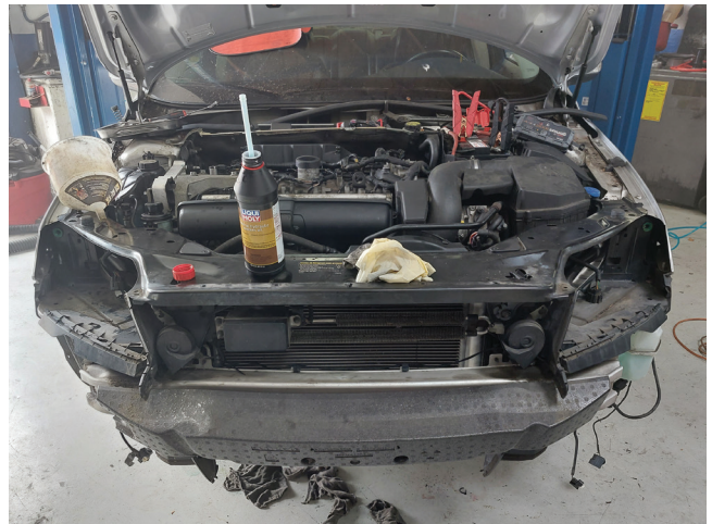
When you pull off the bumper cover, be sure to store it in a safe location with the painted side up to avoid scratching the paint.
