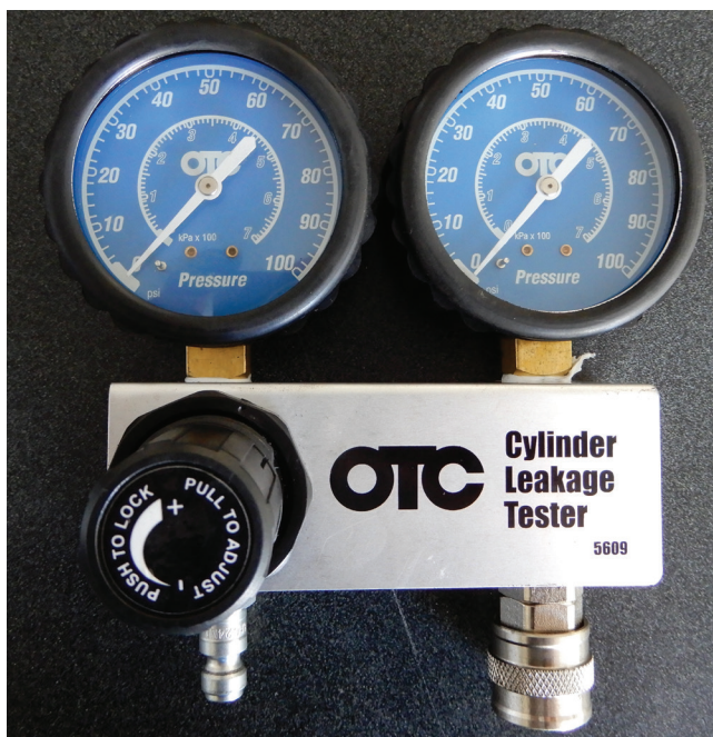
Leakdown tester used to check cylinder leakdown
