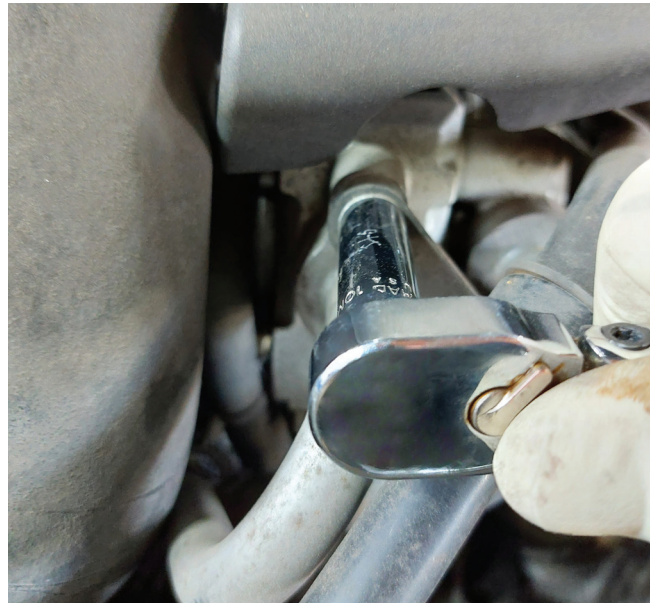
It's a tight fit behind the radiator, so quarter inch tools are the ticket.
