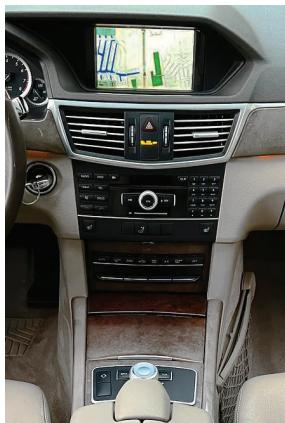
The NTG4 system was offered in both Audio 20 and COMAND versions, the control panels are nearly identical. The larger display screen seen here means this is a COMAND version, while the Audio 20 version has a somewhat smaller screen. Note the presence of the controller knob near the ashtray.
