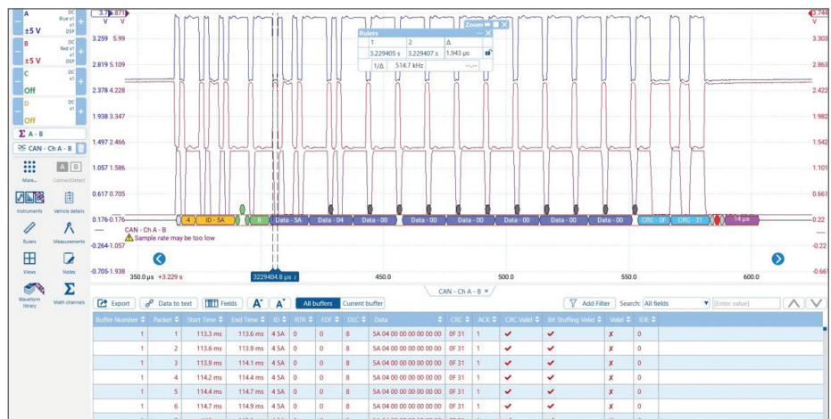
Figure 6: Here we see the decoding procedure where failed packets are sorted by message ID for fault isolation.
