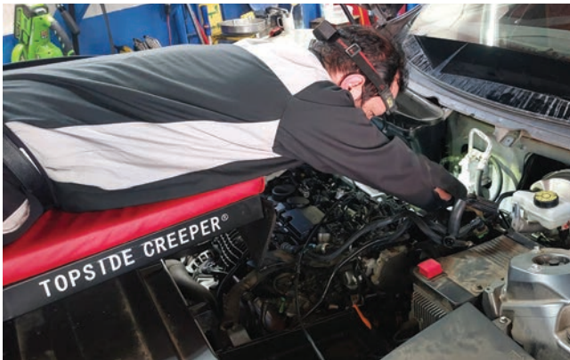
Using a top side creeper to access back of the engine compartment
