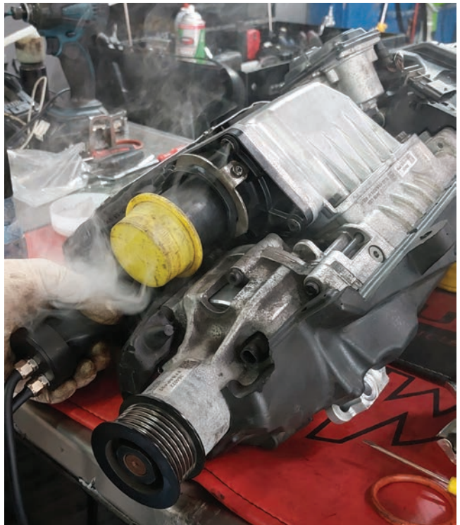
A smoke check of the supercharger assembly when it is first removed will show most of the leaks.
