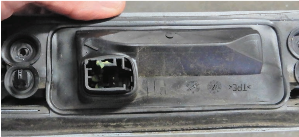
Trunk handle switch assembly removed from vehicle
