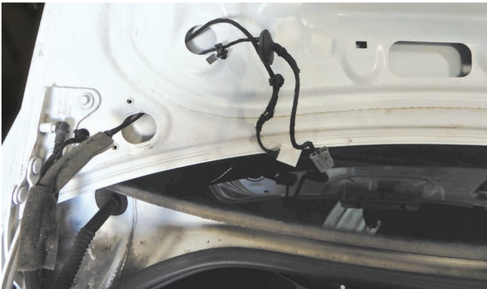
Trunk lid with inside trim removed and exposing wire harness
