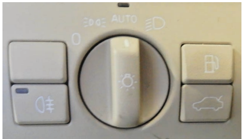
Switch for opening trunk on dash at light switch panel
