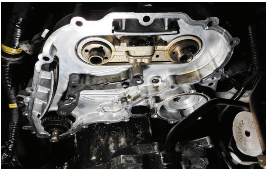
Inner timing cover that needs to come off and replace inner gasket
