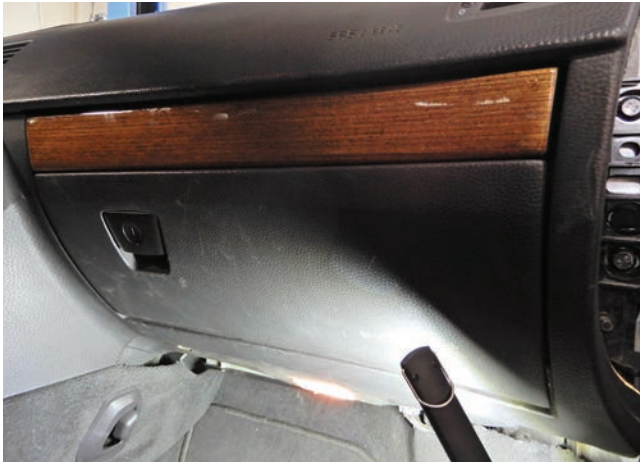
Glove compartment that needs to be removed
