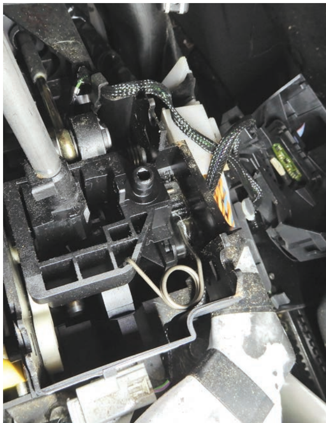
Shifter assembly with shifter kit removed
