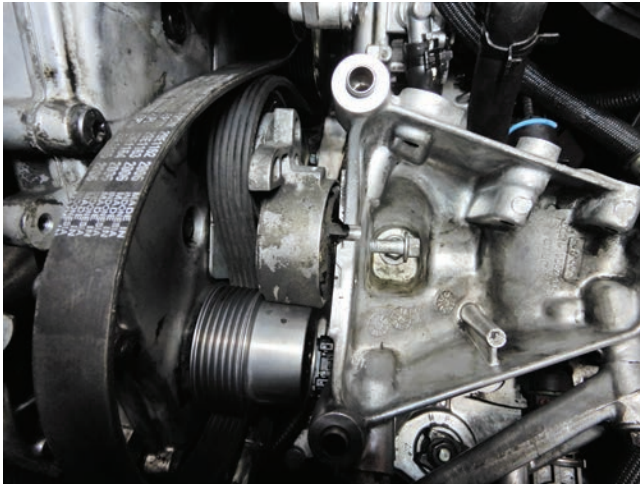
Drive belt tensioner that needs to be removed
