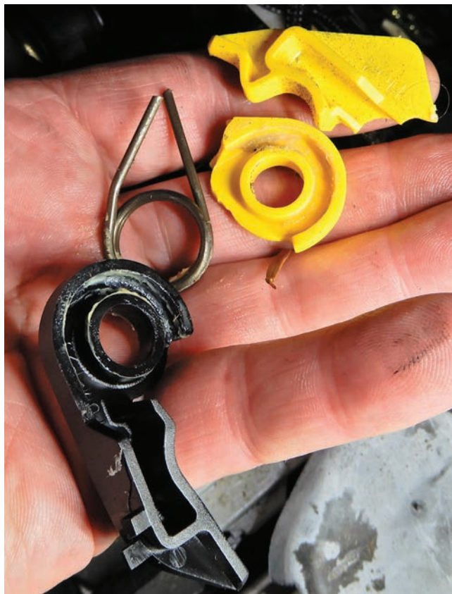
Broken shifter kit that will need to be replaced
