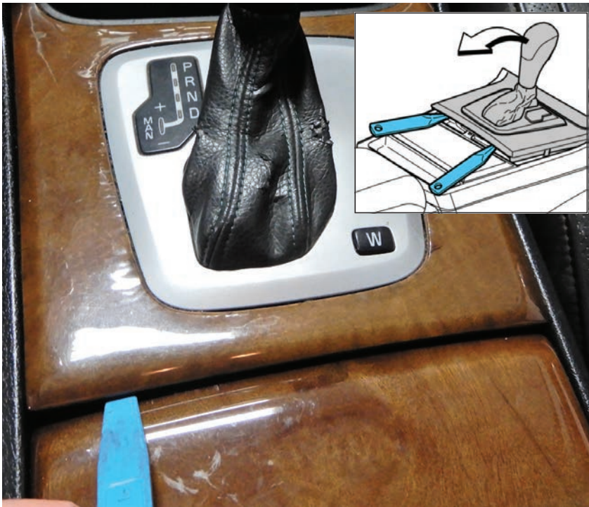
Trim tool used to remove trim at shifter shaft
