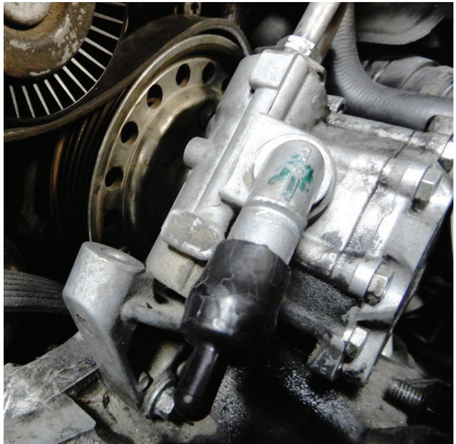
Power steering pump connected to water pump
