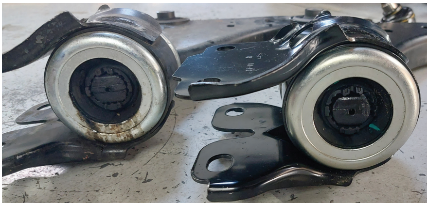
Here's an old leaking hydro control arm bushing compared to new bushing.
