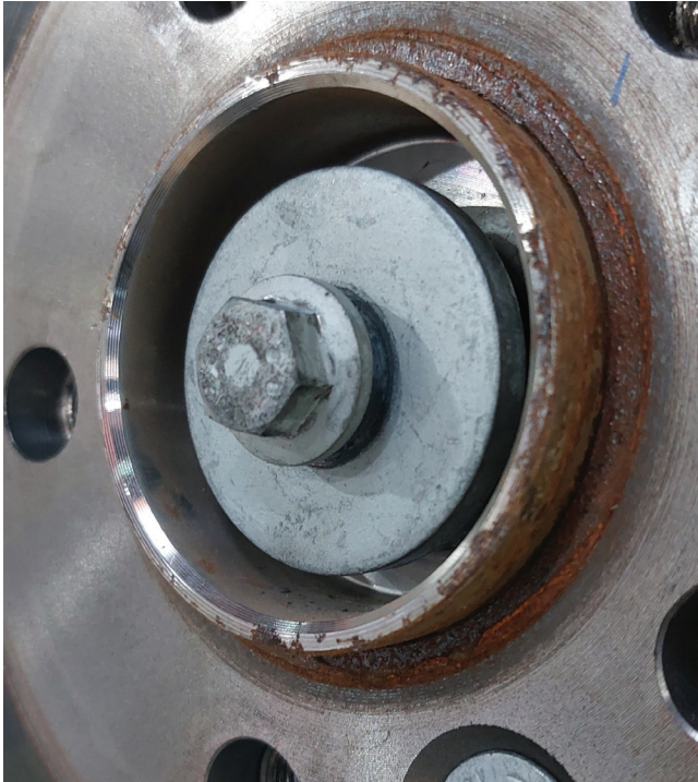
Loosen the axle bolt to make it easier to pop out the ball joint.
