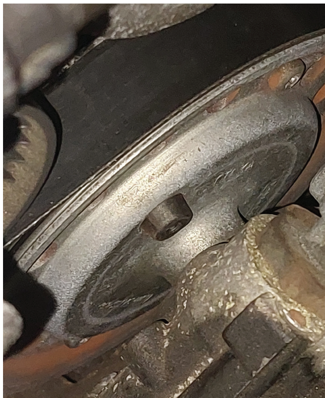
Water pump coupler pin showing through power steering pulley
