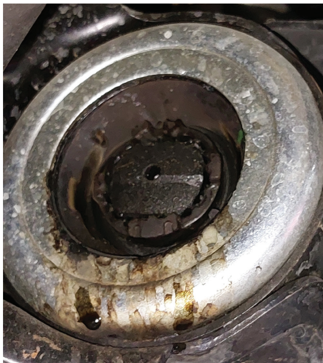
Leaking lower control arm bushing
