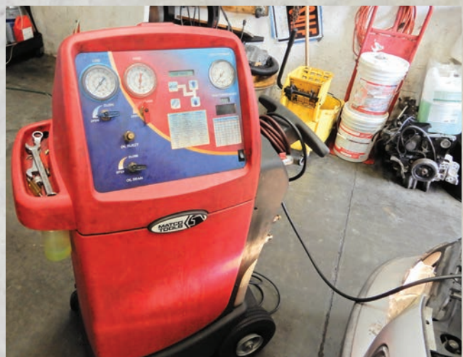
Air conditioning machine hooked up to vehicle at low and high side connectors under hood of vehicle
