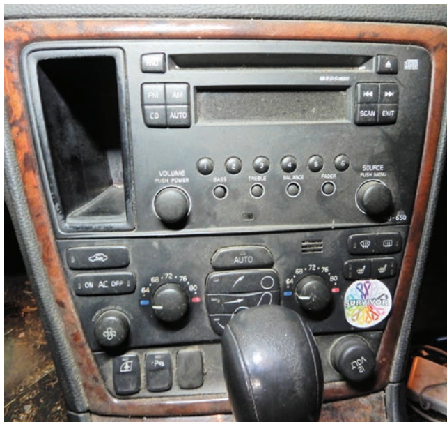
Radio and climate control unit that needs to be removed from vehicle
