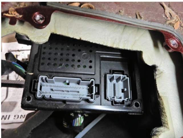
The two T25 torx screws that need to be removed at frame to CEM
