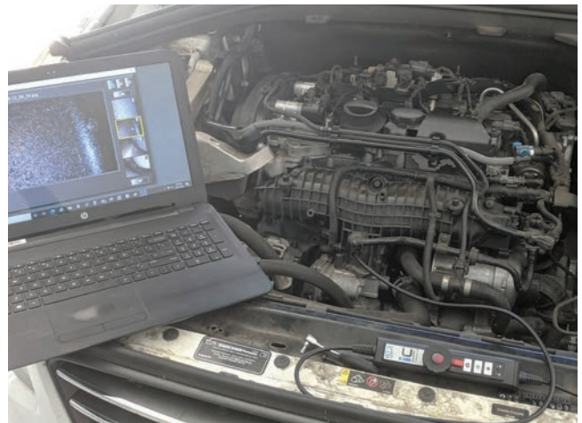
Checking valves with borescope
