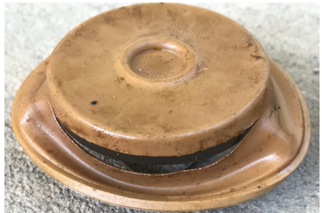
Torn internal diaphragm in the oil separator
